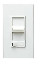
Decora CFL Slide Dimmer can help. It's able to detect the high- and low-end dimming capability of a CFL, and it adjusts power output to improve the bulb's performance and dimming range. The device works with a wide range of dimmable CFLs (as well as incandescents). It costs about \$20.
