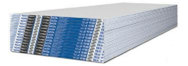
Light and Stiff. Easi-Lite gypsum board weighs up to 30 percent less than standard gypsum board and has a high-strength core that allows it to span 24-inch oncenter ceiling joists without sagging, says CertainTeed. The company also claims that the material is easy to score and snap and is made with 100 percent recycled face and back paper. It's sold in 4-foot-wide sheets in 8-, 9-, 10-, and 12-foot lengths for \$7 to \$10 apiece.
