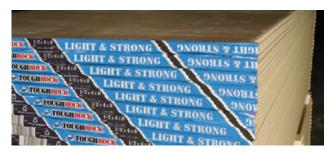
Hard Rock. Compared with standard drywall, *ToughRock Gypsum Board* is less likely to crack, sag, or absorb moisture, the maker says. It also weighs 25 percent less and is Greenguard-certified for low VOC emissions. The product is suitable for interior walls and ceilings, veneer plaster base systems, and fire-rated assemblies. A <sup>1</sup>/<sub>2</sub>-inch-by-4-foot-by-8-foot sheet costs about \$8.
