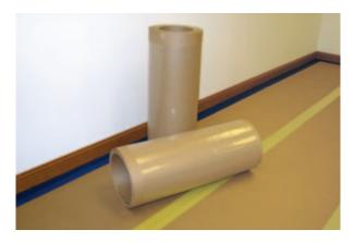
Floor Saver. According to the maker, FlexBoard does as good a job of protecting finished floors as hardboard does, but it's a lot easier to handle and store. The 45-mil-thick product is water-resistant, nonstaining, and vapor-permeable, and it's made from recycled materials. It can be laid over vinyl, laminate, wood, concrete, stone, marble, and tile; after a job it can be reused or recycled. A 32-inch-by-50-foot roll costs \$30, a 100-foot roll \$50.
