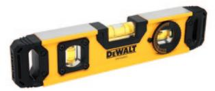
Versatile Torpedo. With the new DWHT43003, DeWalt has given the lowly torpedo level a significant upgrade. The tool has an extruded aluminum body with machined edges, and solid block vials that are guaranteed accurate to within 0.0005 inch/inch. One edge is V-grooved and fitted with magnets for work with metal and pipes. Other improvements include a magnified center vial and a rotating end vial with an angle scale on one side and a roof-pitch scale on the other. The level costs about \$25.
