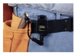
Tool Tether. The Gear Keeper Retractable Lanyard (model RT4-5601) features a rotating belt clip and a 36-inch tether that's suitable for tools weighing up to a pound. (A beefier model for 2-pound tools is also available.) Prices range from \$27 to \$35. Separate connectors that allow users to swap out individual tools cost \$5.
