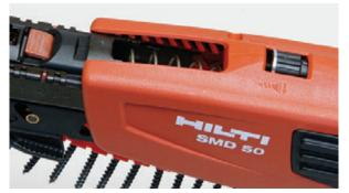
To convert to autofeed, you install the Phillips bit included with the magazine (top) and then snap on the magazine in one of 12 positions. You remove the magazine by pressing the release buttons and pulling it off (center). The magazine's depth gauge is set by pushing the orange button on top and sliding the gauge until it shows the desired screw length; it's fine-tuned with the thumbwheel (bottom).
