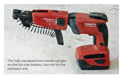
To set the magazine's depth gauge, you push a button on top and slide the gauge until it indicates the desired screw length, fine-tuning if necessary by turning a thumbwheel. You can remove the magazine in a second by squeezing the two release buttons and pulling it off.
