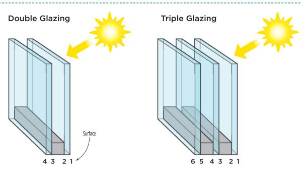
The placement of low-E coatings on multi-glazed windows may vary with the climate zone. Glass surfaces are identified by number, beginning with outermost or "weather" surface. It is always designated as #1, the inner surface of the outer pane is surface #2, and so on. In glazing with suspended films rather than internal glass, the film surfaces are numbered the same way.
