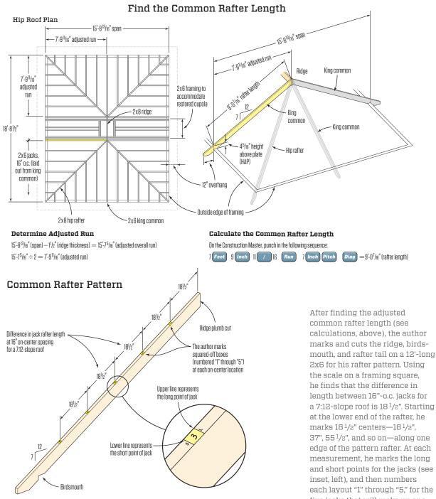
and short points for the jacks (see each layout "1" through "5," for the five jacks that will make up one side of a corner of this hip roof.
