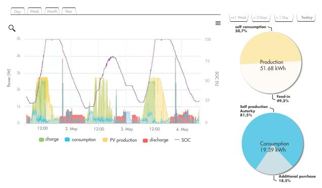
**Knowledge is power.** The user interface for Sonnen's battery bank and grid-tie control system supplies an up-to-the-minute display of the home's energy use, energy production, battery charge, and battery discharge. This example, taken from a grid-tied house with grandfathered net metering, shows how the home's battery charges up in the day and discharges at night.
