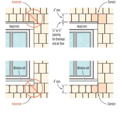
When you're shingling around windows, exposure should be no less than 4 inches for the courses above and below the windows. Be sure to leave ample clearance between the course above the window and the head flashing. For proper drainage, align the shingle gaps with the corners and avoid having shingles that wrap around the corners.
