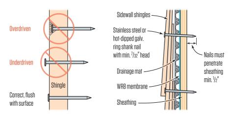
Always drive nails flush to the surface of the shingle. Underdriven nails do not anchor the shingle properly and overdriven nails break the wood. Additionally, always use nails that are the proper length. Remember that nails must go through the layers of shingles, through the drainage plane, and then through the sheathing with a penetration of at least 1/2 inch. Nails for fastening shingles should be either stainless steel or hot-dipped galvanized.
