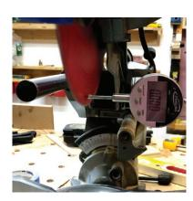
Blade-wobble results were verified by recording the running saw blade in slow motion, and then visually observing if the pin jumped around. Kerf cuts were made in 4-by material and measured with a caliper.
