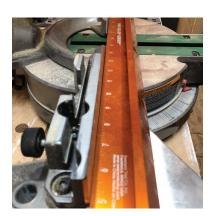
Table and fence straightness was observed using a straightedge.
