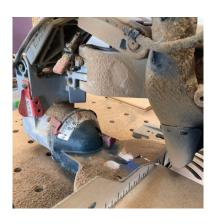
The dust-collection test was conducted using a new 60-tooth Diablo blade in each saw. Consistent numbers of cuts were made in the same material types. Dust was captured in a bag and then weighed.
