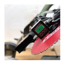
As a matter of course, detents were checked using a digital angle finder with the saws set on a flat, level surface. All saws came in either at exact readings for the respective detent, or within three tenths of it.
