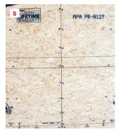
Foam-to-gel glues work on wet or dry wood (2). If fastening sheathing with a nail gun, be sure to use ring-shank or twist-shank nails (3). A stand-up screw gun takes longer to drive each fastener, but is just as fast for the job overall (4). Manufacturers often print the fastener layout on the sheets (5).
