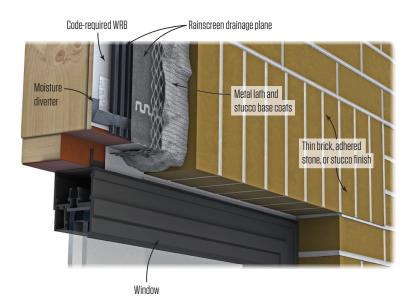
Without continuous exterior insulation, a moisture-diverter channel works like an umbrella over the stucco bucket. This channel should slope at  $^{1}/4$  inch per foot above the rough opening and be integrated with the WRB. It should also extend at least 4 inches beyond each side of the opening to kick the water from the drainage space to the sides of the window opening, where it can drain at the base of the wall.
