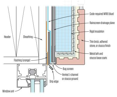
This is the problem: A drainable assembly has nowhere to drain (top). When you are using continuous exterior insulation with thin brick (above), the insulation can kick the assembly outwards far enough to create a drain reveal with thin-brick corner pieces.
