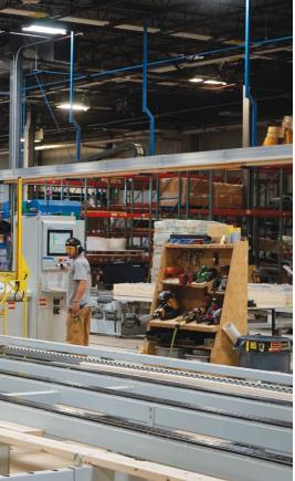
(Facing page) The CNC bridge gantry is equipped with nailers and a router. It travels over the wall on the table, fastening the sheathing to the framing and trimming it to the final panel size as well as cutting out the sheathing for any door and window openings (4).
