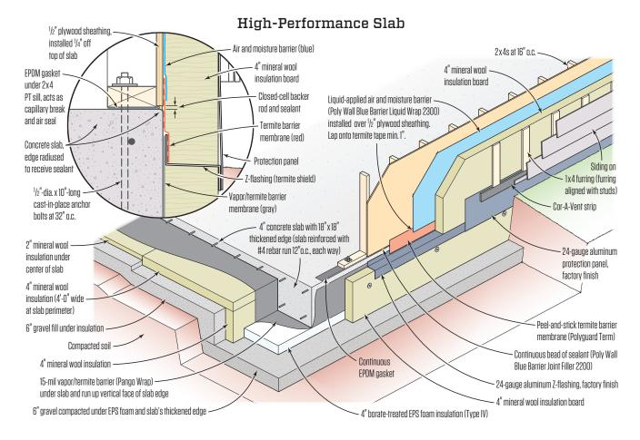
Above is a version of the author's slab detail from a wood-framed house in Marietta, Ga. Here, the author has used a bent metal termite-control flashing integrated into a sub-slab Pango Wrap termite-control vapor barrier membrane. The slab and the wood structure are all contained within the conditioned envelope of the building.
