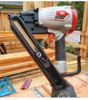
The Max SN438J SuperLocator positive placement nailer has a compact magazine that holds 1½-inch metal-connector nails and allows the gun to fit between joists; an air deflector cap that rotates 360 degrees so you can aim exhaust away from your face; and a swiveling belt hook. Instead of a probe, the tip of the nail is used to locate the hole in the hardware.
