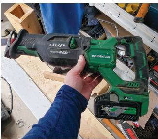
The Metabo HPT MultiVolt reciprocating saw has a brushless motor that can be powered by plugging it into a 110-volt AC outlet or by attaching its 36-volt 4.0-Ah battery. The smooth-operating saw features a variable speed control, straight and orbital cutting modes, and a toolless blade lock mechanism.
