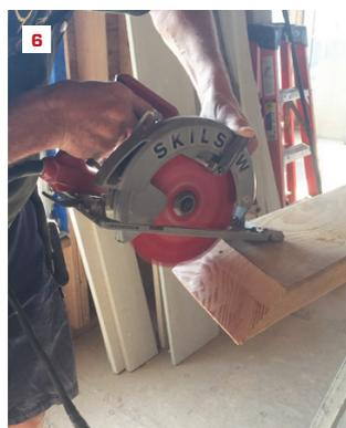
Cut the plumb cut angle with the blade set to the complement of the desired bevel angle and in the opposite direction (1). Following a line marked along the end cut (2), make the next cut with the blade set square and to maximum depth (3). Mark the rest of the cut (4) and make a shallow pass to remove most of the waste (5). Finally, carve down to the line with a series of sliding cuts, moving the saw sideways across the face of the bevel and not taking too much off at once (6).
