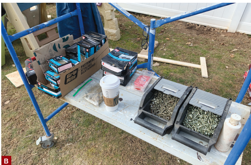
Figure 2. Horizontal surfaces invite being loaded up with random stuff, but a site-built miter saw stand can also double as a valuable work table (A). Even if not needed for working at height, a rolling scaffold offers a convenient spot for storing fasteners and other small items, and it can be rolled to where those items are needed (B).
