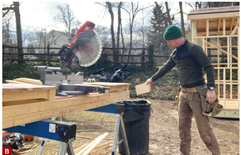
Figure 1. The ability to roll a stack of lumber around instead of moving it board by board contributes to efficiency (A). Placing a trash can to collect offcuts saves the time and energy needed to pick them up off the ground (B).
