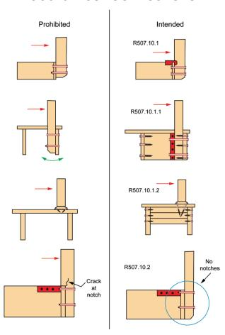
On the left are examples of incomplete guard load paths, while the examples on the right illustrate how blocking, structural screws, and metal hardware can be used to correct those defects by tying framing members connected to the post back into adjacent joists.
