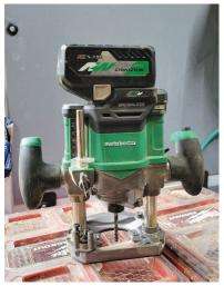
A router fitted with a flush-cutting bit makes quick work of cutting out door and window openings in a sheathed wall (above). Metabo HPT's MultiVolt plunge router comes with collets for both 1/2-inch- and 1/4-inchdiameter bits. It can be powered by its 36-volt battery or be used with an adapter and plugged into an AC outlet (left).
