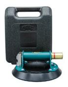
Transporting and installing a large, heavy window is safer and easier with vacuum cups, which clamp onto the glass (far left). Wood's Powr-Grip N4950 8-inch-diameter vacuum cups (left) are rated for 125 pounds and have a redline indicator that signals a loss of vacuum pressure. They come with a carrying case.
