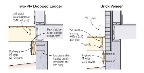
A double-ply dropped ledger may be required to provide adequate bearing for the ends of the deck joists (far left), but this detail requires careful review of the load ratings for the concrete anchors and inspector approval. When there is brick veneer cladding, anchor the ledger to the foundation below the brick ledge and never to the brick itself (left).
