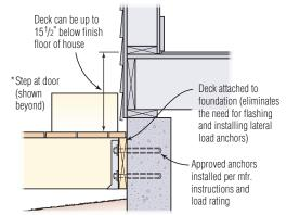
\*Note: the IRC requires at least one side-hinged door with no more than one 73/4" step to a landing. All the other exterior doors of the house can be up to 151/2" down to a landing.
