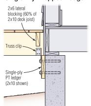
A step (or two) down to the deck is usually needed when a deck ledger is anchored to a concrete foundation rather than to the house framing (far left). Instead of hanging the deck joists from the ledger, installing them so that they bear on the ledger (like a dropped beam) allows the deck to be flush with the house floor framing (left).
