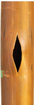
As water freezes in a water pipe and turns to ice, it expands and pressurizes the liquid water remaining in the pipe. Because water is difficult to compress, the pipe will burst if there is no other means for relieving the increased pressure.
