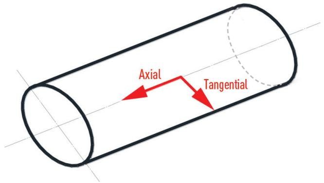
Tangential stress caused by internal pressure in a water pipe acts perpendicular to axial stress and tends to separate a pipe wall in a line parallel to the pipe's center line.
