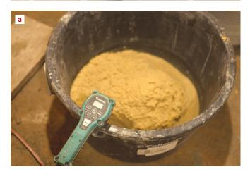
The Collomix AQiX delivers pre-selected dosing quantities from 0.3 to 99 quarts, in 0.1 quart increments. It connects to a garden hose with a standard <sup>3</sup>/4-inch hose coupling (1) and has a battery-powered display (2). It comes with a metal bracket that can hook onto the mixing vessel (3).
