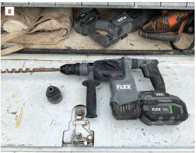
While the Flex FX1551A rotary hammer is designed for SDS-Plus bits, its brushless high-torque, low-speed (0–980 rpm) motor is ideal for driving large drill bits through thick material. Here, the author is drilling a pilot hole through wall framing with a ship auger bit as part of a window retrofit project (1). The battery-powered tool comes with an adjustable side handle, built-in LED lighting, and both an SDS-Plus bit holder and a ½-inch metal chuck (2).
