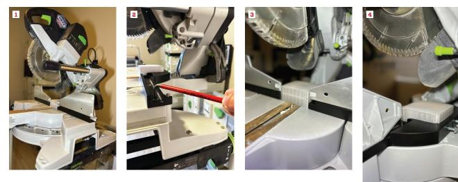
Comprising a black, powder-coated aluminum fence base and a plastic block, the Colliflower Cube system marries easily to a Festool Kapex saw using the saw's existing bolts and holes (1, 2). The Cube fits the fence's throat completely to prevent fly-aways and reduce material tear-out but doesn't impede dust collection or limit depth of cut (3). Adjustment bolts ensure that the Cube remains aligned with the front of the fence (4).
