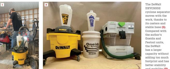
moves with the work, thanks to its casters and stable base (1). Compared with the author's Oneida and Festool units, the DeWalt has a larger capacity without adding too much footprint and has better stability and mobility (2).
