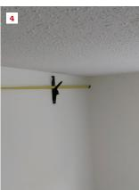
With the crown squared up in the framing square, we can find the distance the crown will sit down from the ceiling (1, 2). A crown hanger is an inexpensive way to hold up crown or a tape measure when you are working alone (3, 4).
