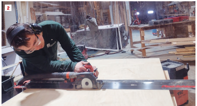
Attached to its crosscut track, the Mafell KSS40 is still light and portable (1). When used with Mafell's 55-inch flexible track, the saw can break down sheet goods or scribe fillers (2).
