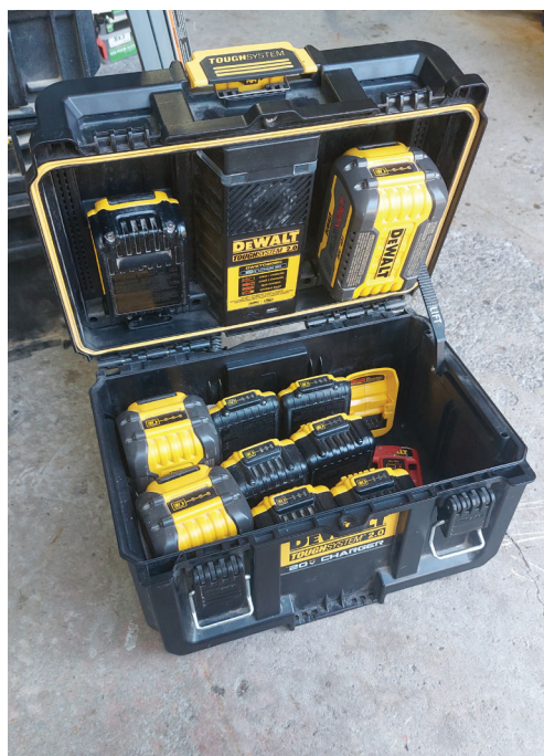
With the DeWalt Tough-System Charger box open, you can see the storage space and the protective lid prop at right.
