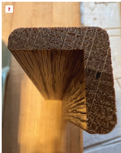
Another example showing a variation in how the grain of a head casing can be centered over the window (6). One leg of any corner molding will have flat grain (in this example, it's the horizontal leg on top), and the other leg will have vertical grain (7).
