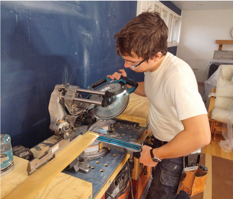
The author can control miter and bevel without having to reach to the back of the saw. The built-in LED light also illuminates the cut area while working (left). Weighing in at a compact 48 1/2 pounds the saw is comfortable to move around the job site (right).
