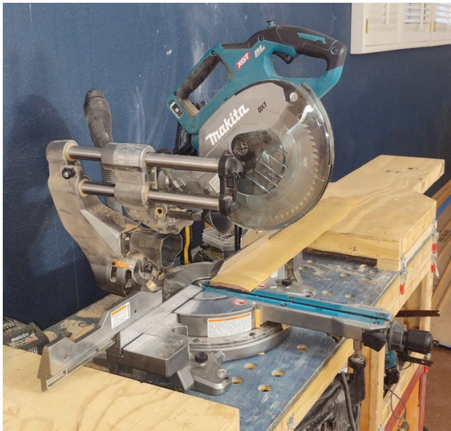
The GSL02Z has a rail-forward system so the saw can be used close to a wall. Note the multi-function front controls (above).
