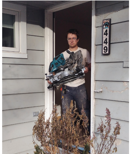
The author can control miter and bevel without having to reach to the back of the saw. The built-in LED light also illuminates the cut area while working (left). Weighing in at a compact 48 1/2 pounds the saw is comfortable to move around the job site (right).
