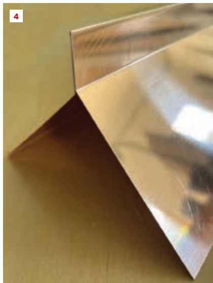
Samples bent by the fabricator show the profiles of the two corner treatments the author uses—the open square (3) and the single fin (4).
